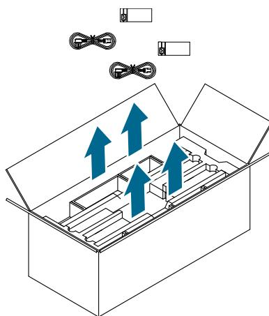
4. Remove two displays, one by one, from the center compartment of the top layer.
